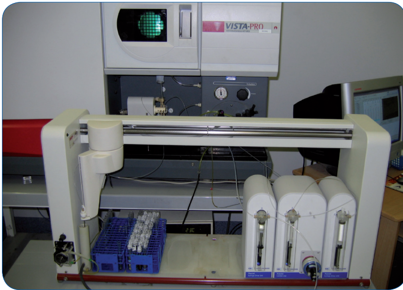
Figure 4: Assist accessory mounted in front of the Varian ICP-OES
