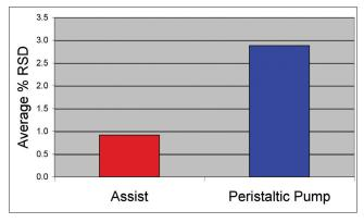
Average RSD for inline dilution using the Assist and peristaltic pump. The dilution factor is 10:1.
