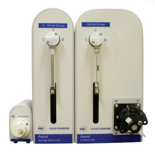
This is the most common system. It incorporates two syringe drives and a Niagara switching valve. It provides for the inline delivery and mixing of the sample with internal standard or diluent.
