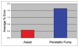
Average error in the measured concentration for 21 elements when the internal standard is delivered inline using the Assist compared with the standard delivery using the peristaltic pump. The ratio of internal standard to sample is 1:10.
