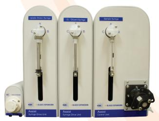
This system is configured specifically for the analysis of wear metals in raw (undiluted) lubricating oils by ICP-OES. It incorporates three syringe drives and a Niagara switching valve. It takes a sample of the oil, mixes it with a diluent such as kerosene and precisely delivers the diluted oil to the ICP spectrometer. It eliminates the need for manual dilutions and dramatically increases the speed of analysis. The cycle time can be under 30 seconds per sample.
