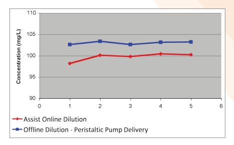
This data shows the accuracy of dilution for five 100mg/L standards. The dilution factor is 10:1 and each point is the average for 21 elements. The data shows that the accuracy of inline dilution using the Assist is significantly better than manual dilution followed by peristaltic pump delivery.
