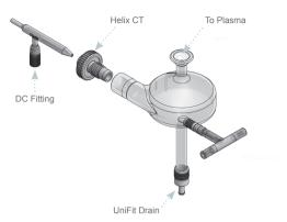
The HydraMist spray chamber uniquely mixes the aersolized sample and liquid to ensure complete formation of the volatile hydride species. Other hyride generation systems rely on a slow liquid/liquid mixing of the sample and reductant which results in incomplete formation of the volatile hydride species and excess hydrogen build-up in the drain. These systems suffer from low sensitivity and poor analytical precision, significantly compromising detection limits.
