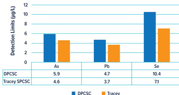
As we can see in Figure 3, when the double-pass spray chamber is replaced with a Tracey™ single-pass spray chamber, detection limits for As improve (reduce) from 5.9 µg/L to 4.6 µg/L, Pb from 4.7 µg/L to 3.7 µg/L and for Se from 10.4 µg/L to 7.1 µg/L. This represents a 22 to 28% improvement in detection limits.
