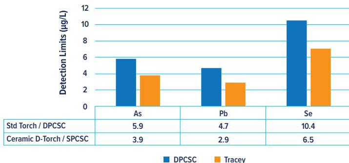
As can be seen in Figure 4, when the standard quartz torch and double-pass cyclonic spray chamber is replaced with a D-Torch™ with ceramic outer tube and a Tracey™ single-pass spray chamber, detection limits are 3.9 µg/L for As, 2.9 µg/L for Pb and 6.5 µg/L for Se, which is a 30% to 40% improvement in detection limits on the standard sample introduction system.
